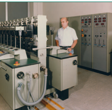
EPZ301 The first electronic reference meter EPZ was constructed. For the first time, an accuracy of 0.1% could be achieved. The EPZ301 was installed into test benches as a unload substandard meter. The max pulse output frequency at nominal load was 9000 Hz. This means that the errors of meters under test could be measured within shortest test times. 1972
