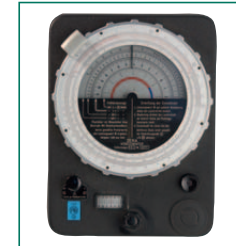
An electromechanical fault indicator type FA3, used to test a dynamic meter. The difference between the set and actual time can be directly read off the dial. 1951
