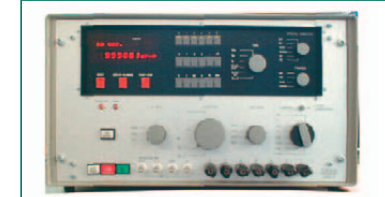
ILM03 A single-phase thermal comparator, for the first time with a measuring accuracy of 0.01%. 1981
