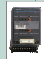
1991 Hybrid meter Electronic meter and electromechanical register (mechanical drum-type register)
