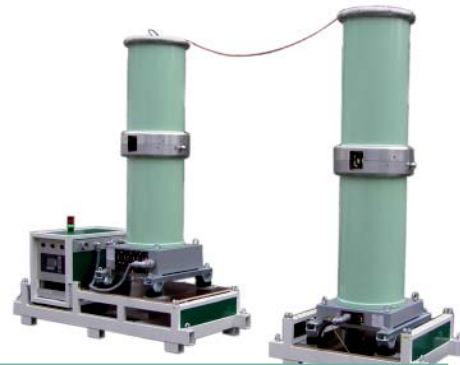
Assembly for high voltage measurement
